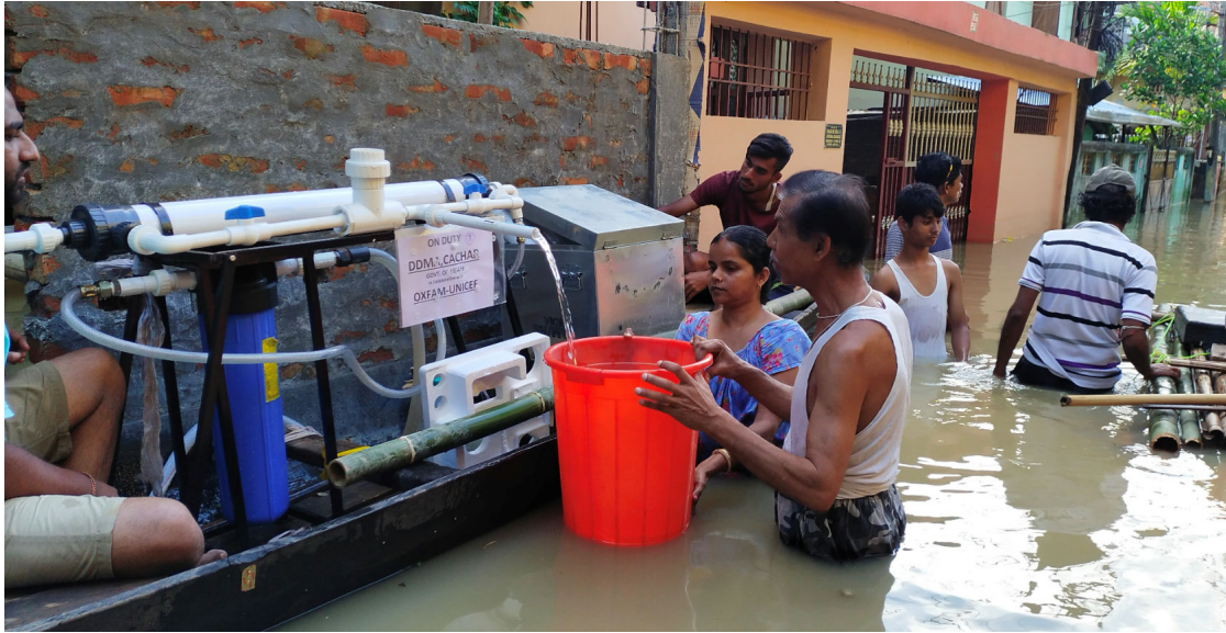
UNICEF and partners provide clean drinking water to affected families in the flooded town of Silchar in the remote district of Cachar, Assam State, using a boat-mounted water treatment plant.
